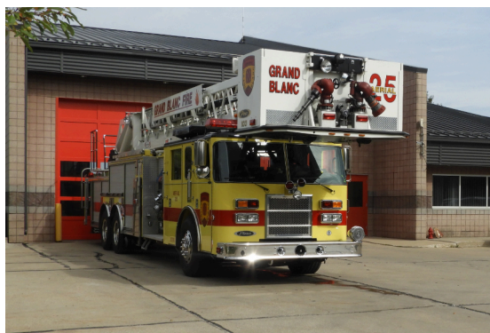
2001 Pierce, 100 ft. Aerial Platform 2000 gpm pump
