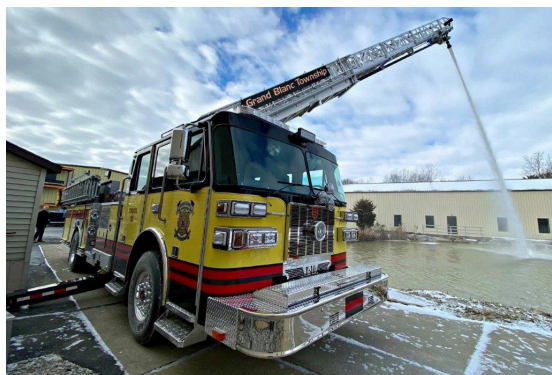
2019 Sutphen, 75 ft. Ladder 2000 gpm pump
