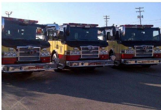
2009, 2010, 2012 Pierce, Pumpers 1500 gpm pump
