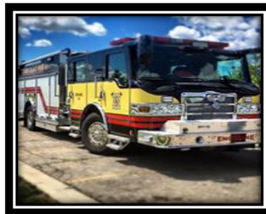
2014 Pierce, Pumper / Rescue 1500 GPM pump and breathing air cascade system.
