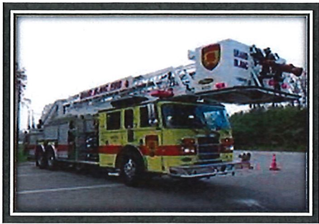
Pierce 2001, 100' Aerial Platform 2000 GPM pump
