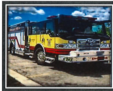
Pierce 2014, Pumper / Rescue 1500 GPM pump and breathing air cascade system
