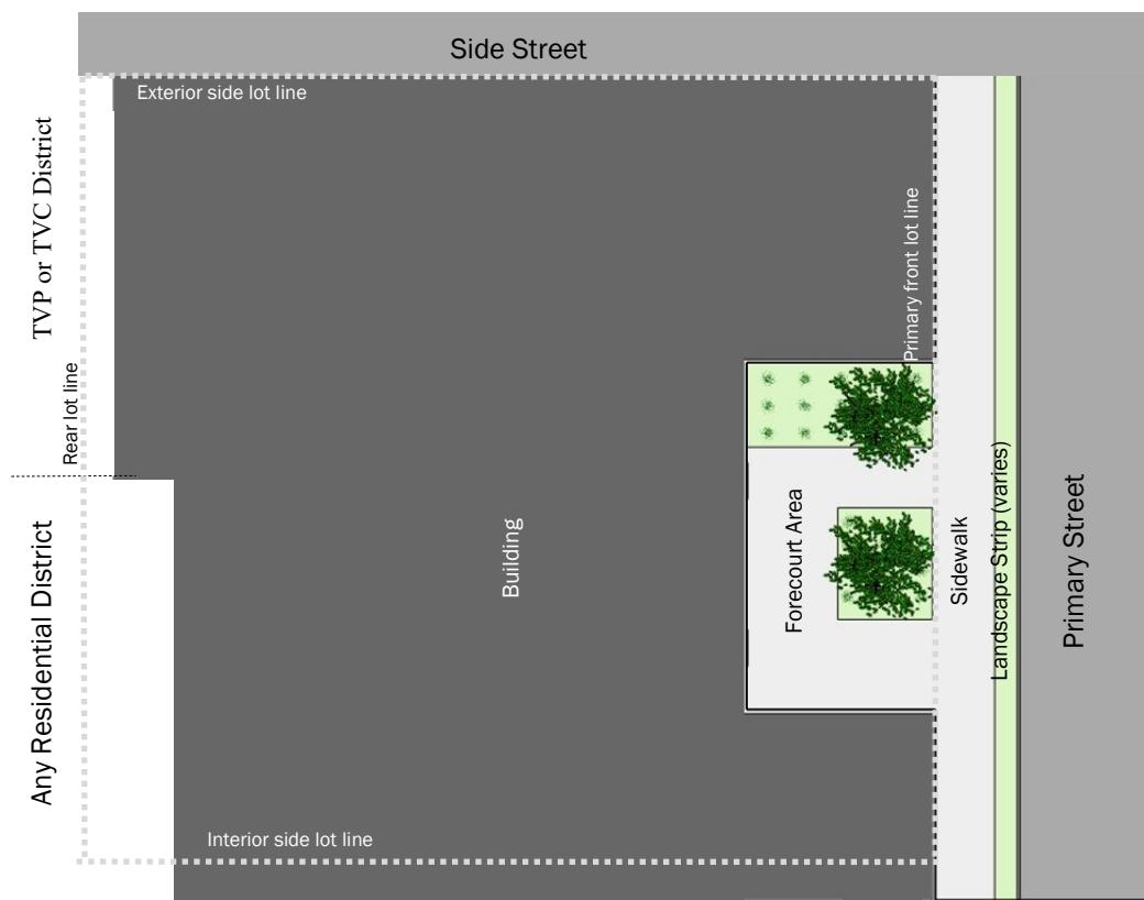
**Frontage Type: Forecourt** These conceptual illustrations show a typical configuration of buildings based on the regulations of this section.
