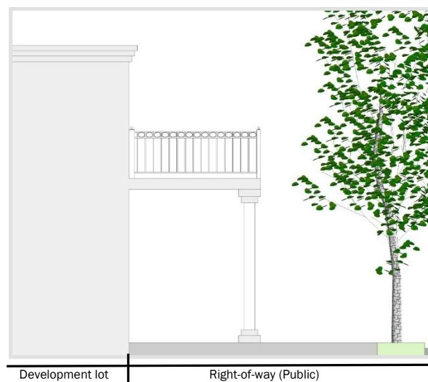
Colonnade may be placed at lot line when the ground floor street-facing façade is set back 10-25 ft.
