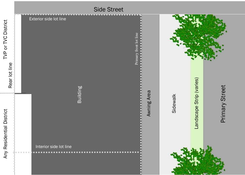
**Frontage Type: Single- and Multiple-Story Shopfront** These conceptual illustrations show a typical configuration of buildings based on the regulations of this section.
